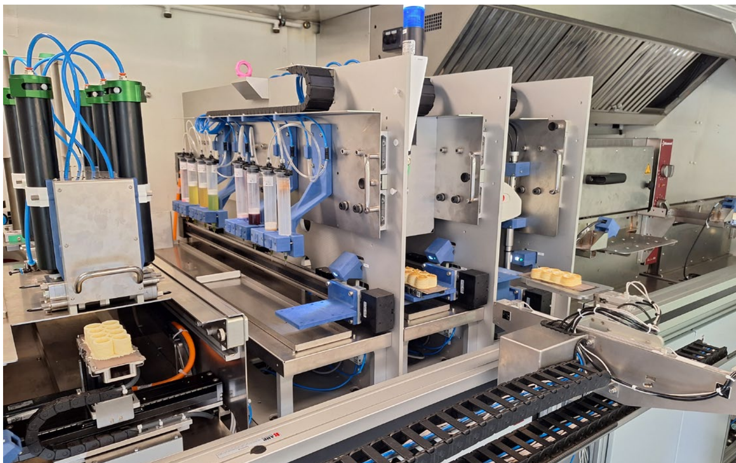
The 3D food printer is made up of several stations. The black cartridges on the left contain dough. The toppings come out of the transparent tubes next to them.
