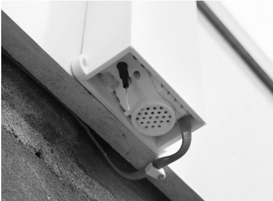
The Heusinkveld sensor in a 3D-printed, durable and weatherproof box • Photo Guy Ackermans
