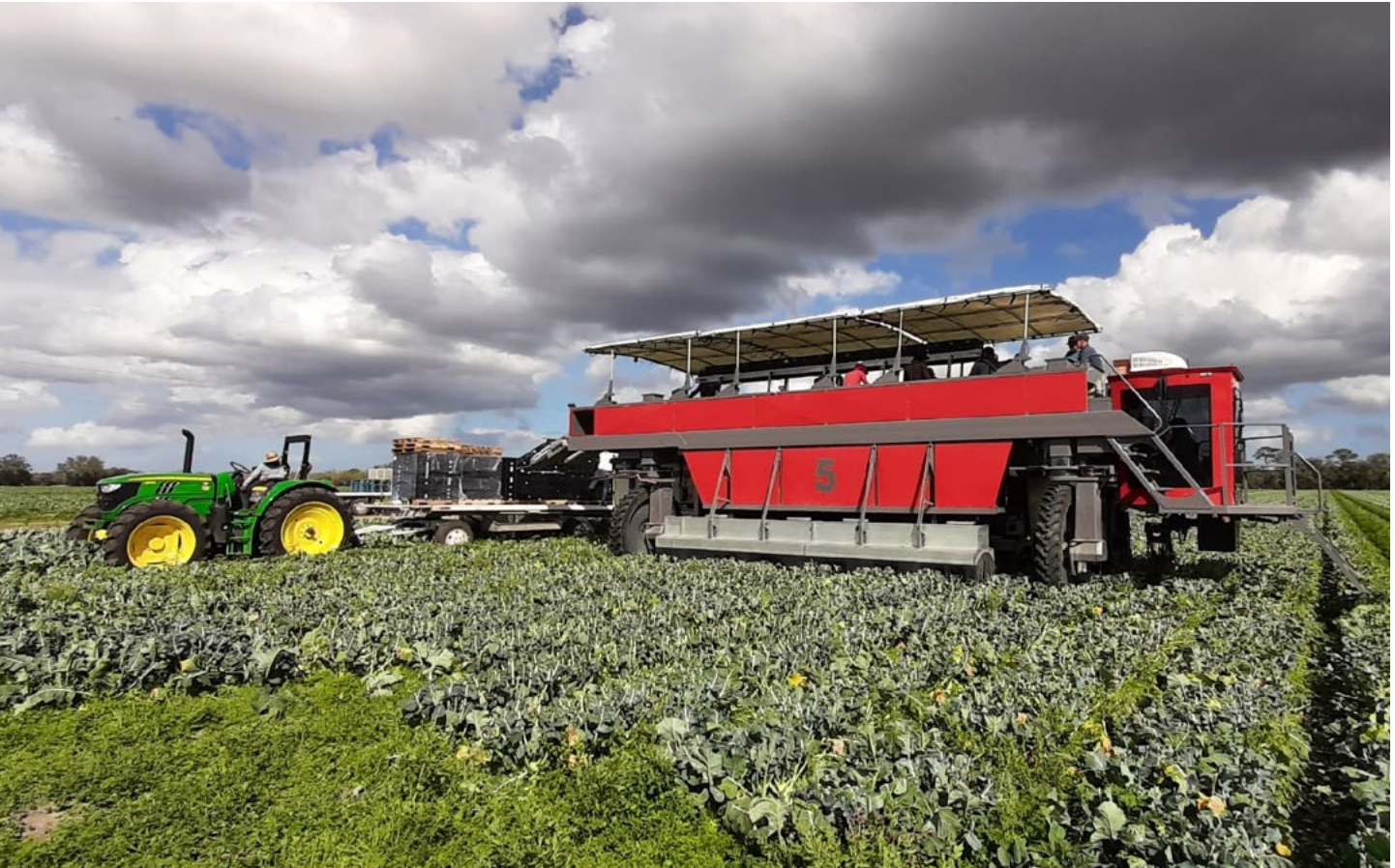
The computer-controlled broccoli harvester. • Photo Pieter Blok
