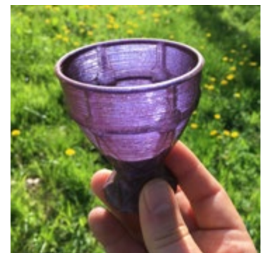
▲ Gold nanoparticles ensure that this cup changes colour depending on the position of the light source.
