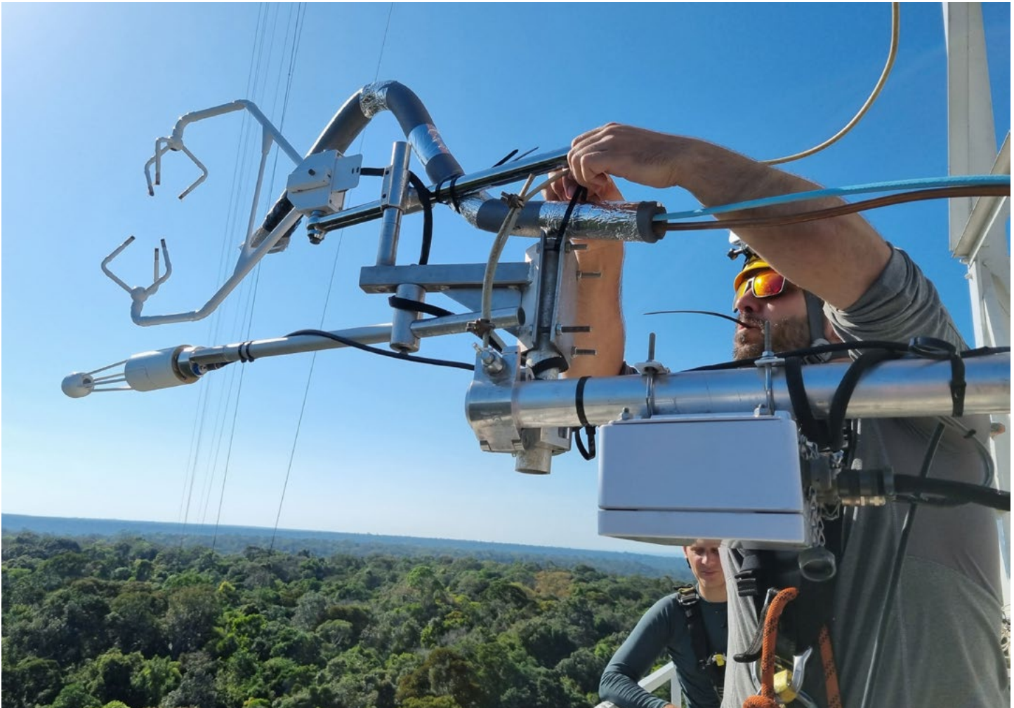
Technician David Bonell Fontas (Utrecht University) sorts out the equipment in the measurement mast. This set-up can measure the transport of CO 2 , H 2 O and their isotope composition. • Photo Oscar Hartogensis
