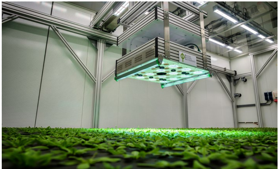
There is complete control over the light falling on the plants in the climate chambers. That allows various aspects of photosynthesis to be studied, as is being done in this photo with the model plant Arabidopsis (thale cress) • Photo Guy Ackermans
