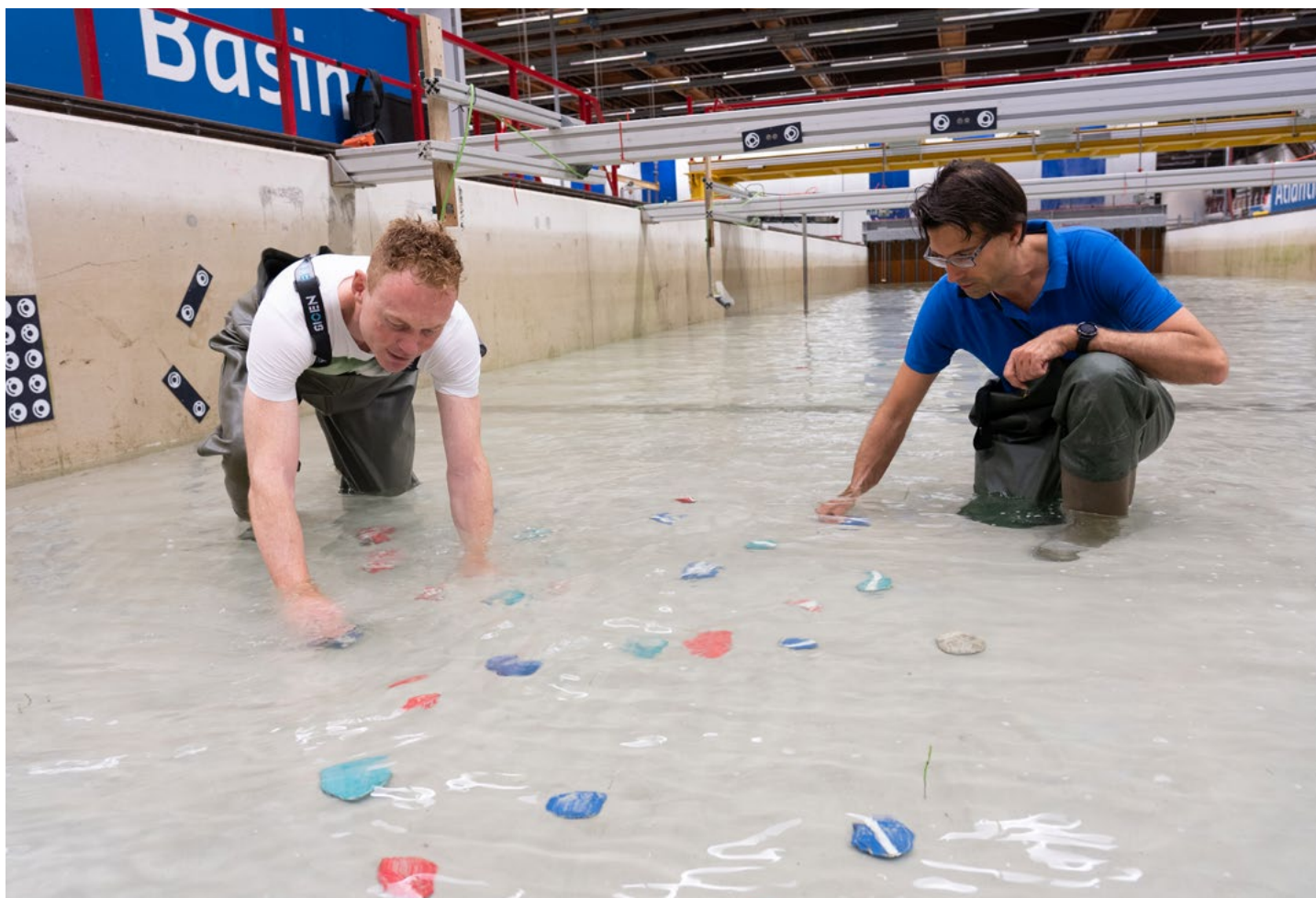
Oscar Bos (left), a marine ecologist at Wageningen Marine Research, and Tim Raaijmakers, an offshore engineering researcher at Deltares, place oysters in a test pool to see how waves affect the oysters' location. Photo Tessa Louwerens
