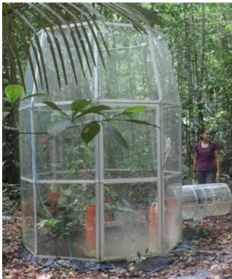
► An Open Top Chamber with which INPA will study how the expected climate change affects the forest. In four of these mini-greenhouses, the trees get extra CO 2 ; the other four form the control group.
