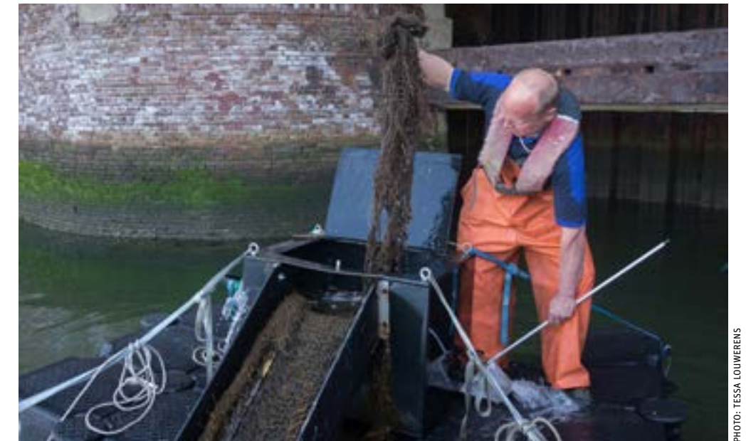
▲ The glass eel detector with the 'climbing wall' being emptied by Bram van Wijk of the Netherlands Fisheries Service (VSN). The North Sea Canal has twelve of these detectors dotted along its length.
