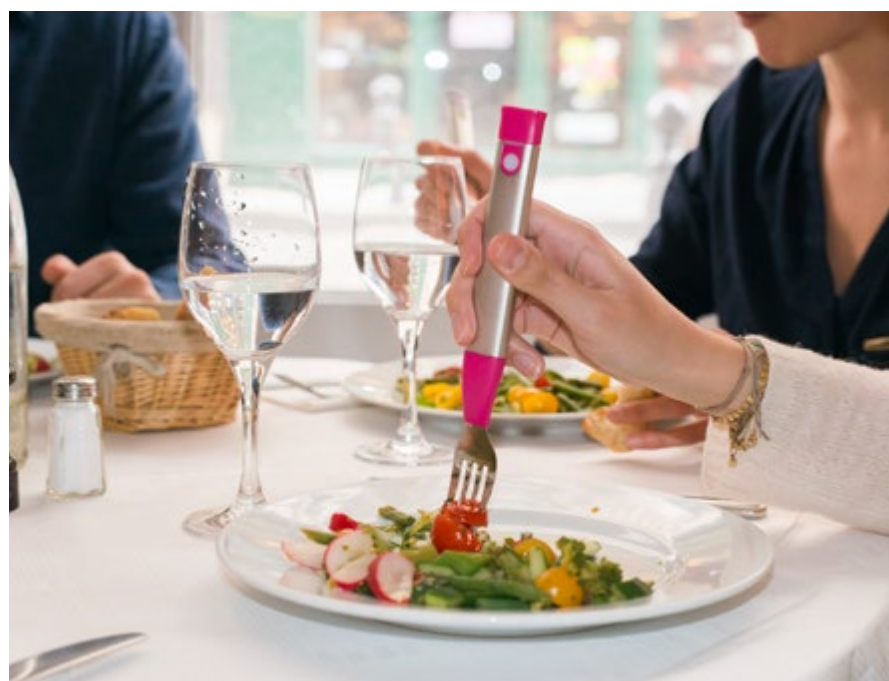
The 10sFork designed by the company Slow Control starts vibrating if the gap between mouthfuls is shorter than 10 seconds.
